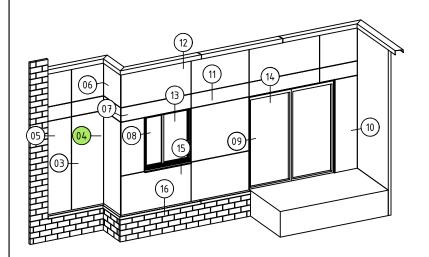
04 PANEL MIDSPAN SUPPORT DETAIL ENCLAD<sup>TM</sup> GRC PANEL
